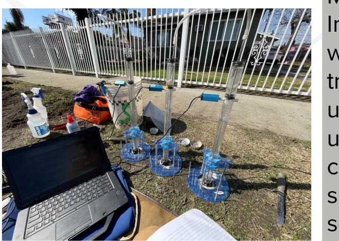
Mini-Disk Infiltrometers adapted with pressure transducers were used to measure unsaturated hydraulic conductivity at the surface and top of the second horizon.
