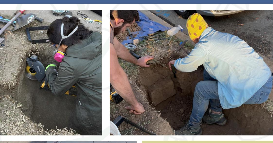
Monolith Monoliths are intact soil trays collected to analyze the structure and natural pores of the soil
