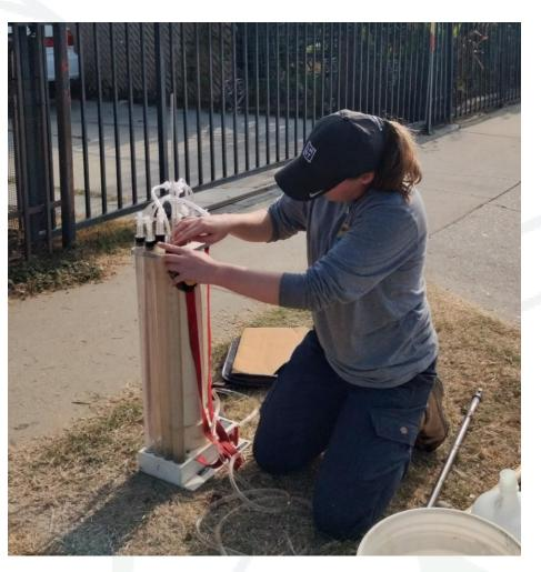
We measured saturated hydraulic conductivity at 2 depths: around 50 cm and 100 cm using an Amoozemeter.
